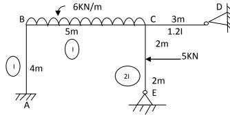
Q.10 Analyze the frame using moment distribution method, EI = constant
