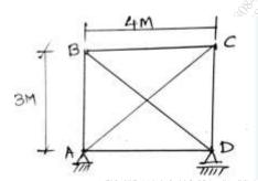
Q.5 Draw SFD, BMD for the beam shown in fig below by using SLOPE DEFLECTION METHOD. If 15 support B sinks by 2.50 mm. take  $I=3.5 \times 10^7 \text{ mm}^4$ ,  $E=200 \text{ KN/M}^2$
