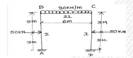
Q.7 Find the end moments of the members of the portal frame as shown in fig by using MOMENT DISTRIBUTION METHOD.
