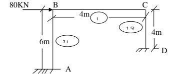
Q.4 A pin jointed rectangular truss is as shown in fig. the members AD is least to be added and is short by 5mm. Find the forces in all the members when it is forced into position. Take  $E = 210 \, GPa$ . Figures in the bracket indicate cross sectional area of the members in cm<sup>2</sup>
