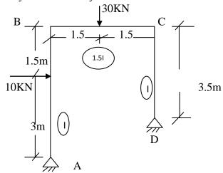
Q.9 Analyze the portal frame as shown in fig. by using moment distribution method.
