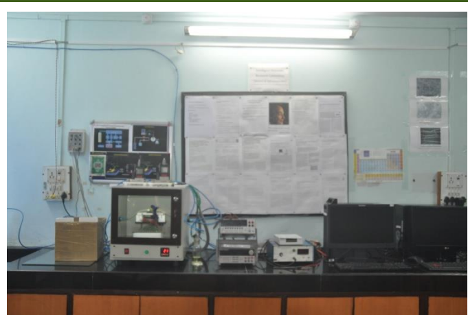
Indigenously Designed & Developed Dynamic Gas Sensing Setup
