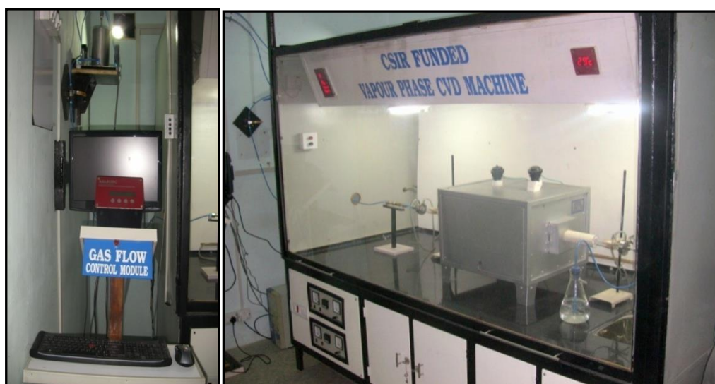
(L) Control console and (R) Mother unit of Semi Automatic Vapour Phase Chemical Vapour Deposition Machine for synthesis of MWNTs and SWNTs (not in vapour phase); [Design, Materialization and commissioning team: Dr. Kunal Datta, Dr. Prasanta Ghosh, Professor Mahendra D. Shirsat]
