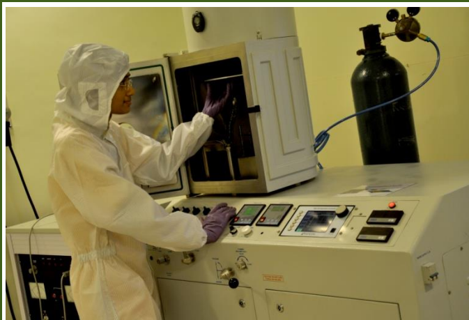
Indigenously Designed Class 10000 Clean Room for Micron level Structure Fabrication
